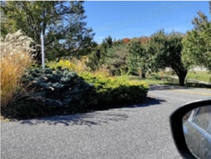
Photograph 30 Art installation blocking sight distance for vehicles travelling south when turning right onto Cumberland Road from Bland Street
